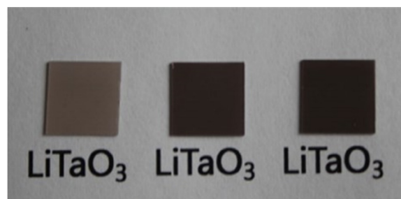
Figure 8. Unrestored LiTaO 3 sheet (left), reduced LiTaO 3 sheet (right, middle). Reprinted with permission from Ref. [81]. Copyright 2020, Springer Nature.
