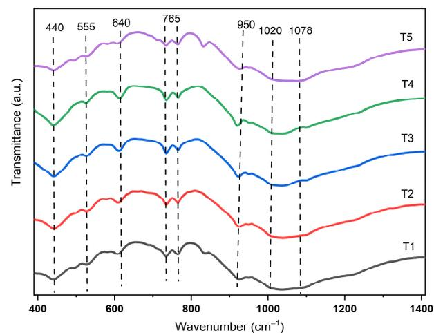
**Figure 3.** FT-IR spectrum of lithium aluminosilicate glass-ceramics with different  $\text{Li}_2\text{O}/\text{Na}_2\text{O}$  molar ratios.
