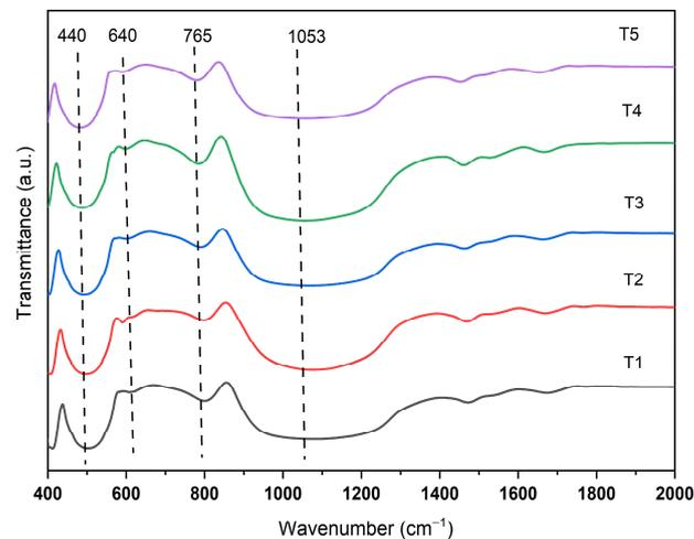
**Figure 2.** FT-IR spectrum of lithium aluminosilicate glass with different  $\text{Li}_2\text{O}/\text{Na}_2\text{O}$  molar ratios.
