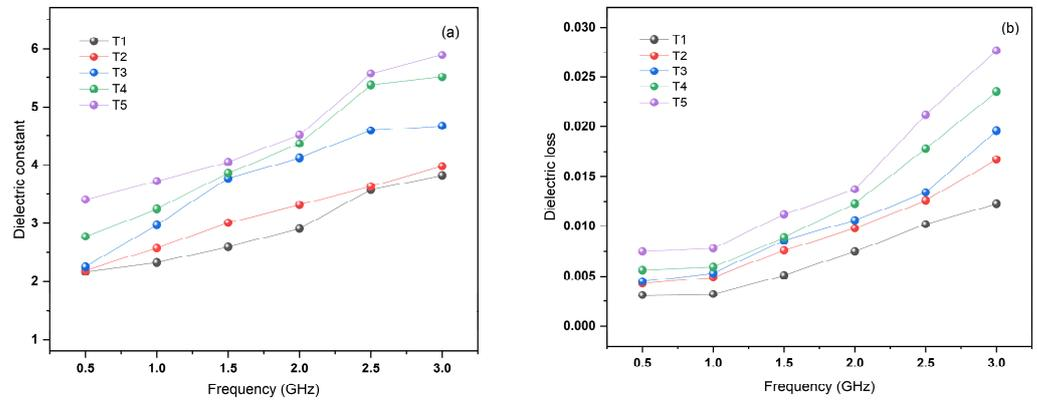
Figure 5. (a,b) dielectric constant and loss of T1~T5 lithium aluminosilicate glass samples.
