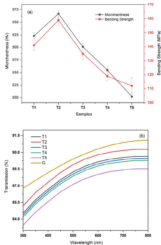
**Figure 9.** (a) Schematic of the flexural strength and microhardness of T1~T5 glass-ceramics; (b) visible-light transmission curve of glass-ceramics.
