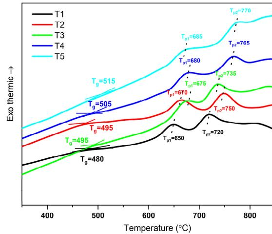
**Figure 1.** DSC curve of lithium aluminosilicate glasses.
