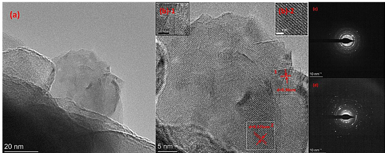
**Figure 7.** (a): Bright-field TEM images; (c,d): SAED patterns of  $\text{Li}_2\text{Si}_2\text{O}_5$  and  $\text{LiAlSi}_4\text{O}_{10}$  crystal; (b): HR TEM images of GCT2 sample; ((b)-1,(b)-2): Schematic diagram of crystal plane spacing of  $\text{Li}_2\text{Si}_2\text{O}_5$  and  $\text{LiAlSi}_4\text{O}_{10}$  crystal.
