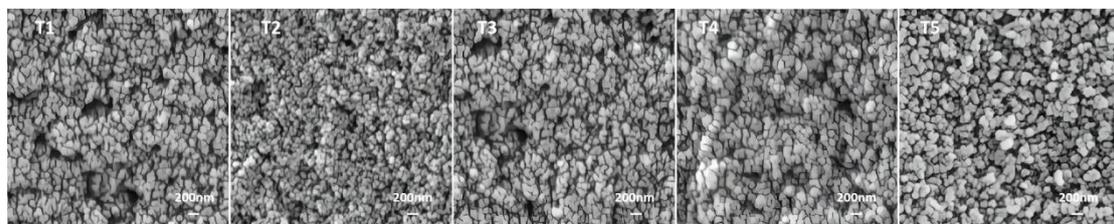
**Figure 8.** FESEM images of T1~T5 lithium aluminosilicate glass-ceramics.
