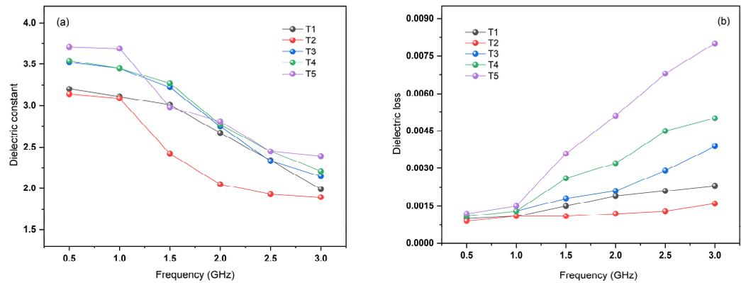
Figure 6. (a,b) dielectric constant and loss of T1~T5 lithium aluminosilicate glass-ceramics.
