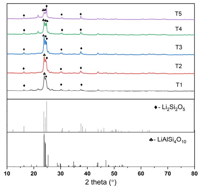
**Figure 4.** XRD pattern of T1~T5 lithium aluminosilicate glass-ceramics.
