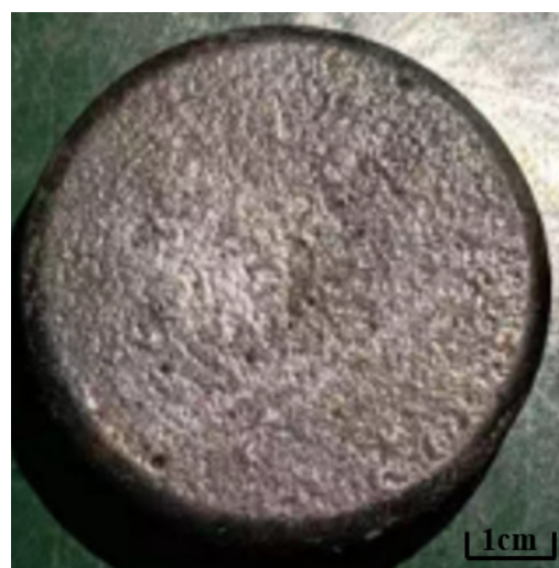
Figure 2. The pre-melted slag sample.
