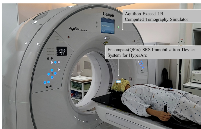
Figure 1. Simulation setup using the encompass SRS immobilization device system for HyperArc treatment on an Aquilion Exceed LB simulation CT scan.
