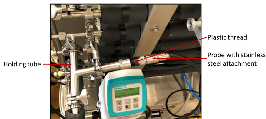
Figure 2. Image of an in-line pH probe inserted within the holding tube of a tubular heat exchanger [51].
