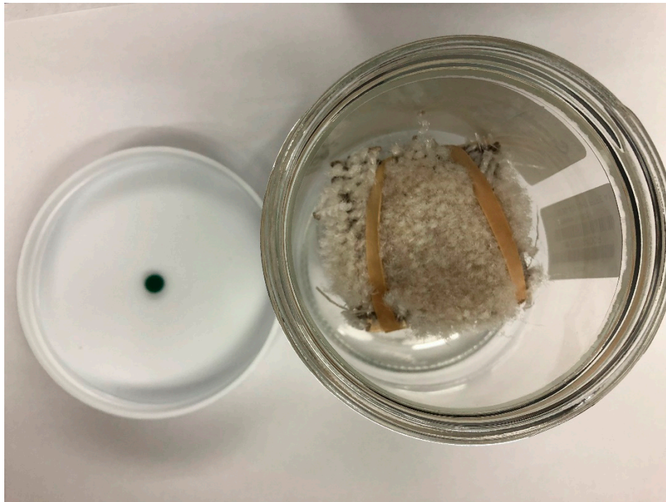
Figure A5. The picture shows the test carpet and subflooring specimen with or without treatment inside the 500 mL glass jar. The carpet specimen was tied with the specimen subflooring using a latex rubberband. Thermogreen half-hole septum in the white plastic screw top was used to insert SPME probes inside the headspace. The inside of the white plastic screw top was lined with PTFE.
