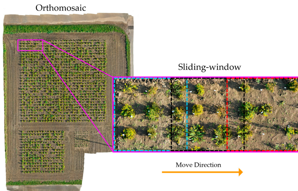
Figure 6. Sliding-window strategy used to process large-scale orthomosaics. Each image chip measured 2048 \times 2048 pixels, with a 10% overlap between adjacent chips. Dashed boxes of different colors represent distinct image chips that scan the entire orthomosaic using a sliding-window approach.
