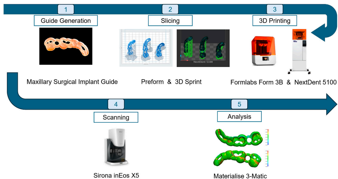
Figure 1. Digital workflow for comparing SLA and DLP 3D printing technologies. The process includes five main steps: (1) surgical guide generation, (2) slicing, (3) 3D printing, (4) scanning, and (5) analysis. Each step is standardized to ensure accuracy and reproducibility.
