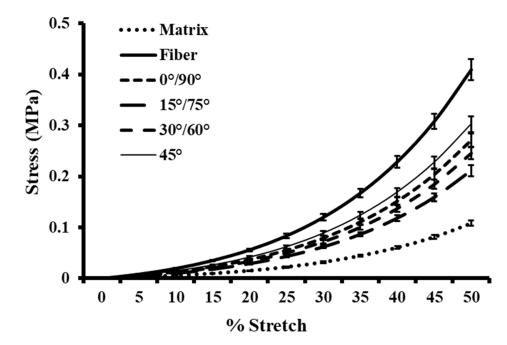
Figure 7. Stress analysis of one-layer anisotropic synthetic skin grafts.
