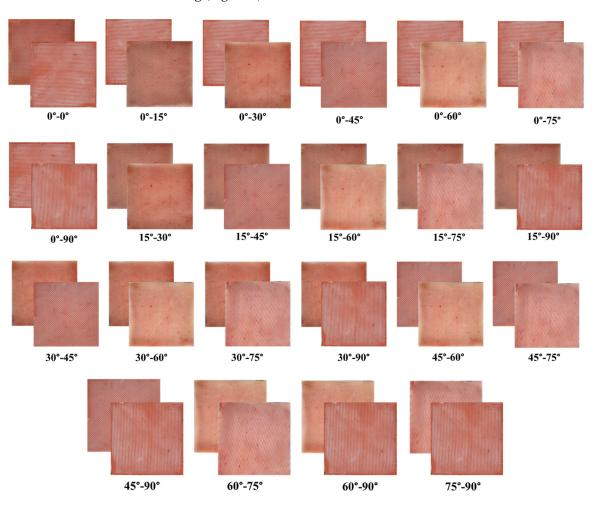
Figure 3. Two-layer anisotropic synthetic skin with varying fiber orientations.
