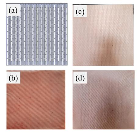
**Figure 4.** Schematic of the development of anisotropic synthetic skin grafts with (**a**) 3D-printed graft meshing slits. (**b**) Anisotropic synthetic skin fabrication; (**c**) projection of slit patterns on synthetic skin; (**d**) resultant synthetic skin grafts.
