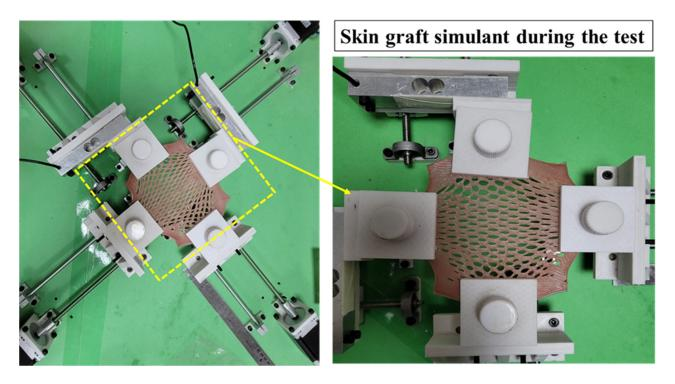
Figure 5. Schematic of biaxial testing setup with attached synthetic skin graft.
