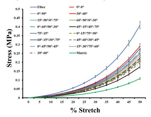
Figure 8. Stress analysis of two-layer anisotropic synthetic skin grafts.
