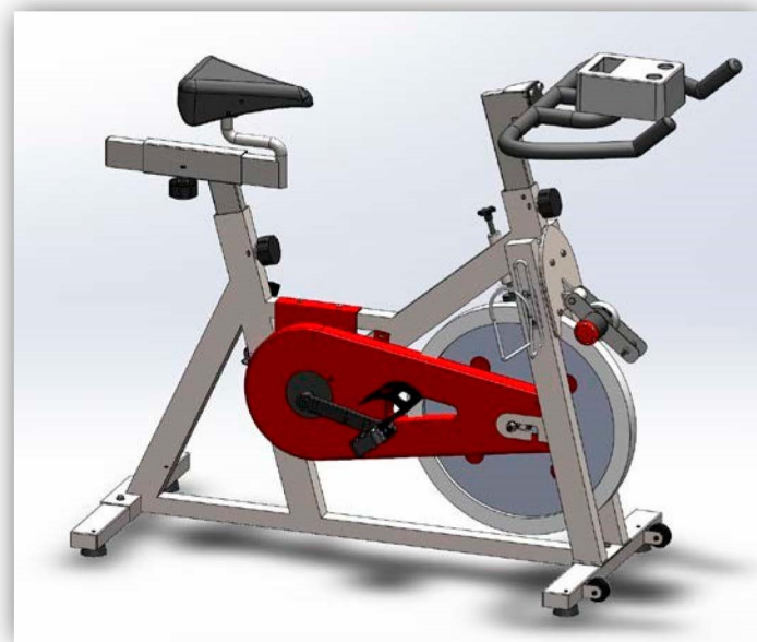
Figure 1. CAD model of a spin bike with an RC motor attached to the flywheel.
