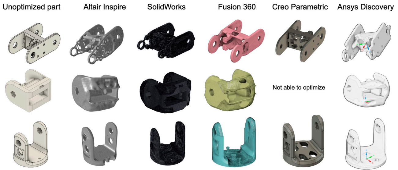
Figure 5. Topologically optimized robot parts per platform. First row: forearm. Middle row: wrist, bottom row: shoulder.
