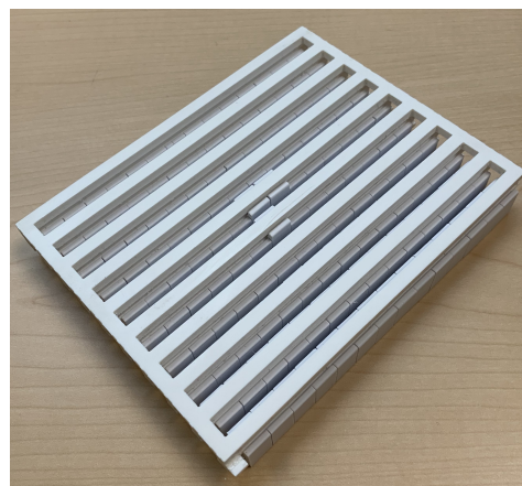
Figure 4. Bottom of part of a prototype of the base where three switches can be seen in their triggered positions.
