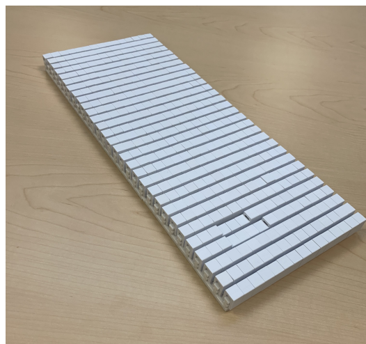
Figure 5. Prototype to be used in the pilot sensitivity study (15 cm × 36.8 cm × 2.2 cm). Seven sensors in the lower left are shown in triggered positions.
