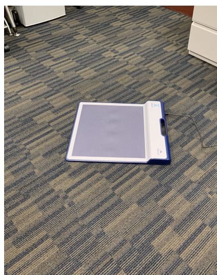
Figure 6. The TekScan MobileMat on the low-pile office carpet where the pilot study was conducted.
