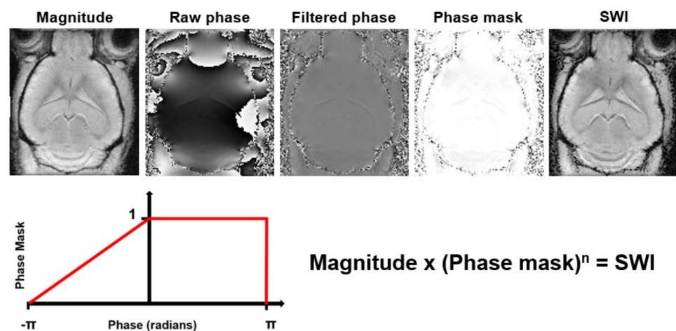
**Figure 7.** Processing steps to generate Susceptibility Weighted Images (SWI) from magnitude and phase data. The raw phase data are filtered to remove low frequency fluctuations. Then, a phase mask that scales the filtered phase images to a range from 0 to 1 is created. This phase mask is then multiplied several times ( $n$ ) with the magnitude image to generate the SWI with enhanced contrast.
