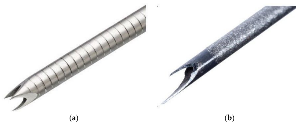
Figure 1. Photographs of (a) a 22G Franseen needle (Acquire™) and (b) a 22G Fork-tip needle (Shark Core™). (a) Franseen needles are made of cobalt–chromium and have a crown-shaped tip with three symmetric prongs. (b) Fork-tip needles are made of stainless steel and contain a nitinol stylet. The device has a multifaceted opposite bevel tip incorporating two sharp prongs of different lengths.
