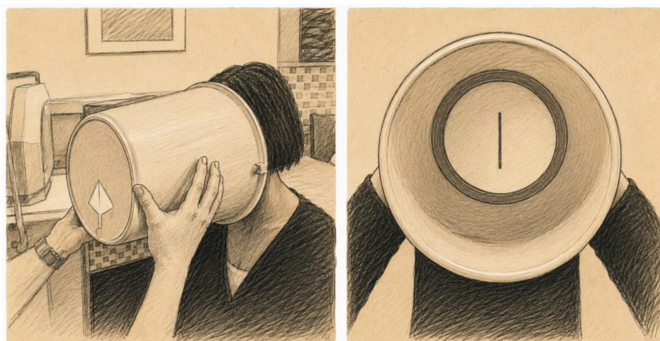
Figure 2. Bucket Test setup for the assessment of subjective visual vertical.
