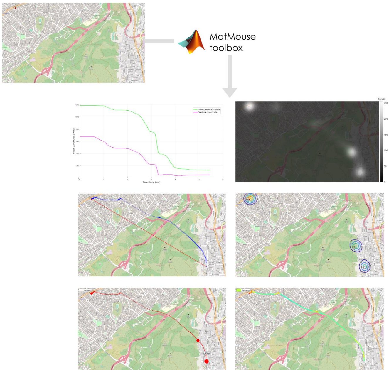
Figure 1. Different ways to visualize and/or quantify the same raw (experimental) data of mouse trajectory produced by the MatMouse toolbox [15] during a task-based map-reading procedure.
