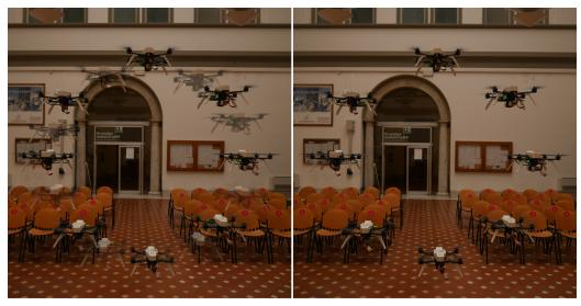
**Figure 11.** Circular mission task: the right image shows the UAV that correctly tracks a circle with a diameter of 1 m and a constant speed of  $0.1 \, \text{m/s}$ . In the left image, the positions taken by the UAV during the execution of a second lap of the trajectory have been superimposed "in transparency". As it is possible to observe, the trajectories followed by the drone are perfectly reproducible.
