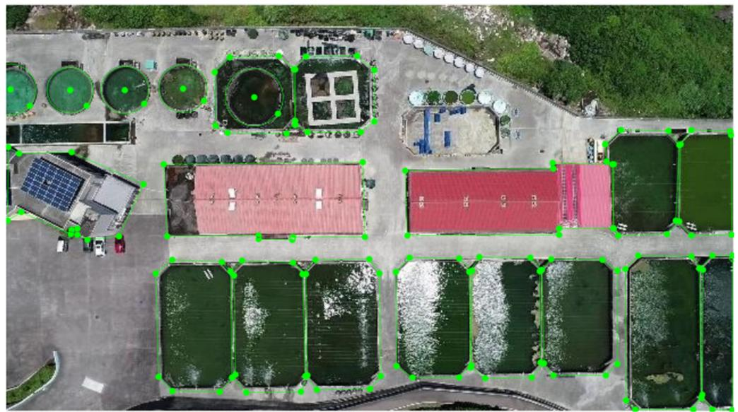
**Figure 7.** Aerial view of in-land aquaculture site with scene modelling with detected objects such as fish pen, cages and house for site surveillance.
