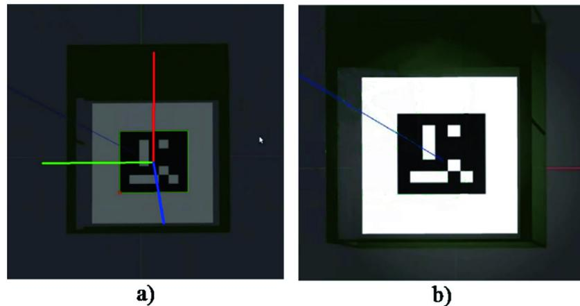
**Figure 4.** ArUco markers used for precise landing with (a) and without (b) the backlight turned on [44].
