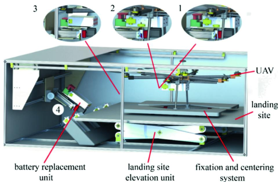
**Figure 3.** Fixed docking station with its subsystems from [44]. The labels (1–4) show the battery replacement mechanism in operation.
