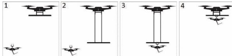
**Figure 17.** Concept of a multirotor UAV transportation system [75]. The numbered labels (1–4) in the figure show in which order are the individual landing stages happening.
