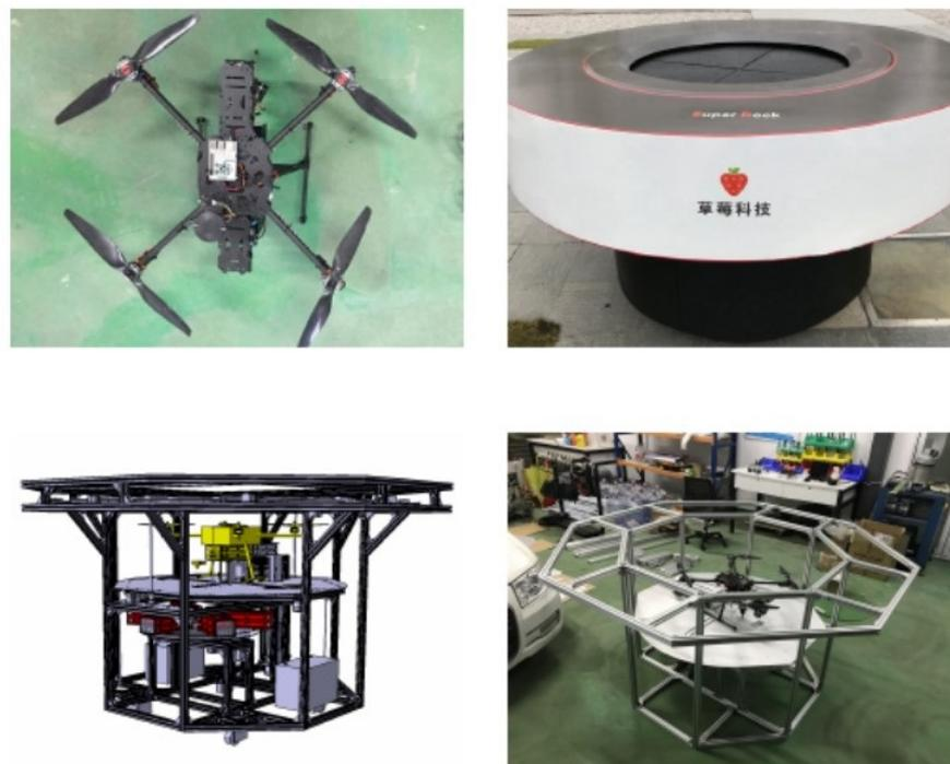
**Figure 5.** Battery replacement docking station from [39]. In the figure, the used UAV is displayed as well as the docking station final version. Furthermore, the design CAD view and the construction phase of the docking station are displayed.
