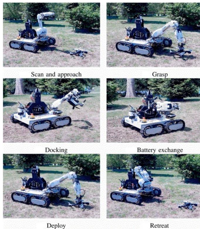
Figure 13. Operation of the proposed UGV-UAV system from [72].
