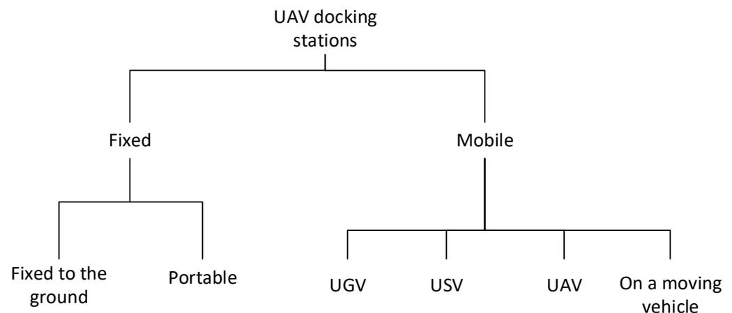
**Figure 1.** UAV docking stations classification.
