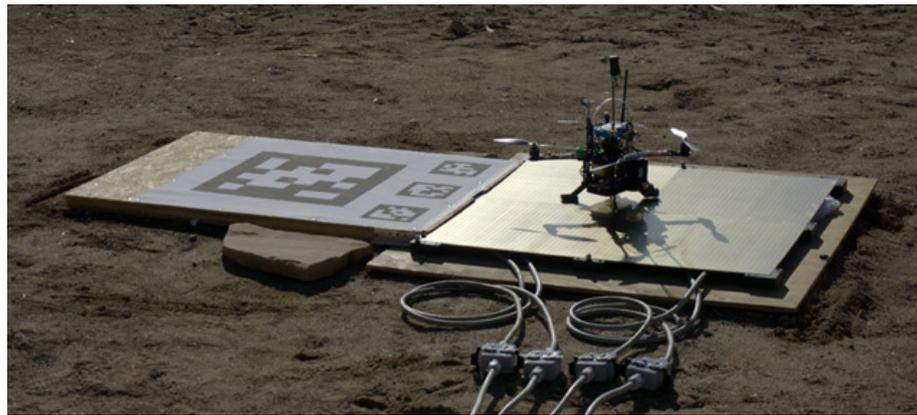
**Figure 10.** Docking station with recharging pad with the custom made UAV from [31]. In the figure, the QR codes used in the approach and landing phase can be seen.
