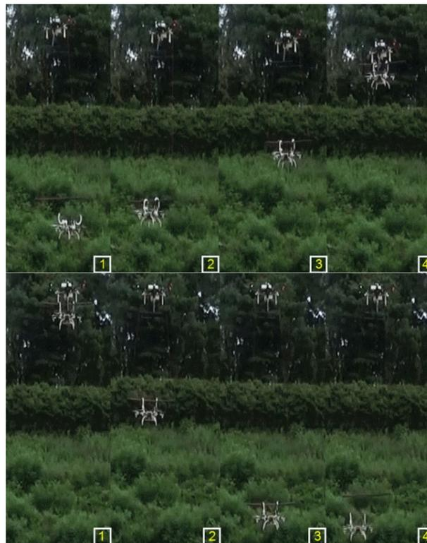
**Figure 18.** Multirotor UAV docking station [75] in operation. The numbers in the picture show all the different landing stages during a test. The first series of figures (1–4) show the approach and docking of the UAV while the bottom figures (1–4) show the un-docking and the separation process.
