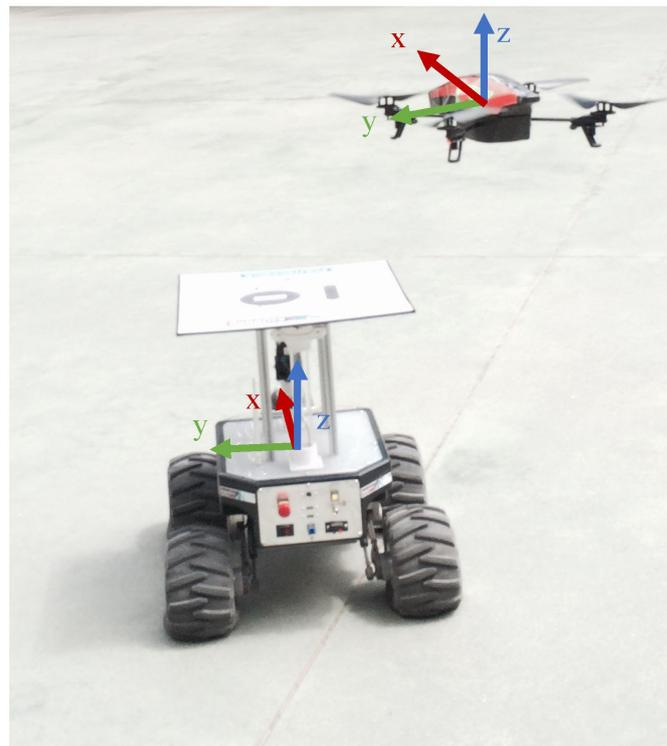
Figure 12. UGV-UAV proposed moving docking station solution from [74].
