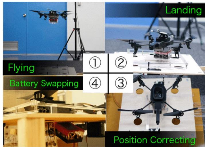
**Figure 8.** Endless Flyer [42], docking station with battery replacement mechanism. The labels in the center show the different landing stages and the order in which they are realized.
