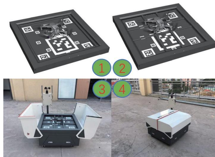
**Figure 11.** Moving docking station with storage system and battery replacement system [65]. Labels in the figure (1–4) show the order in which the active positioning mechanism and storing mechanism take place.
