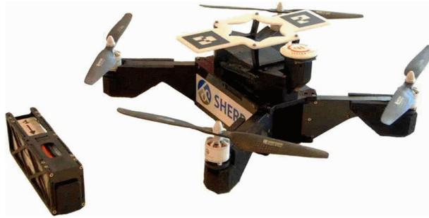
**Figure 14.** Wasp [72]—custom-made UAV with replaceable battery system. All the stages of battery replacing operation are labeled on the bottom of every sub-figure.
