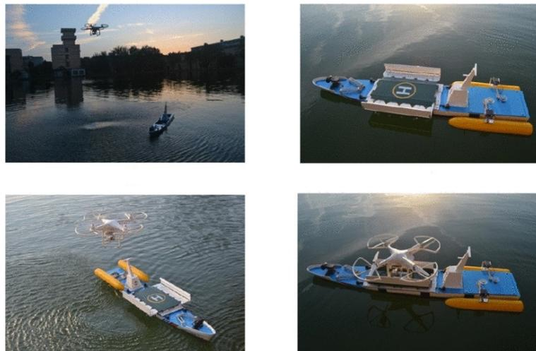
**Figure 15.** USV-UAV landing system proposed in [81]. The whole landing operation is shown.
