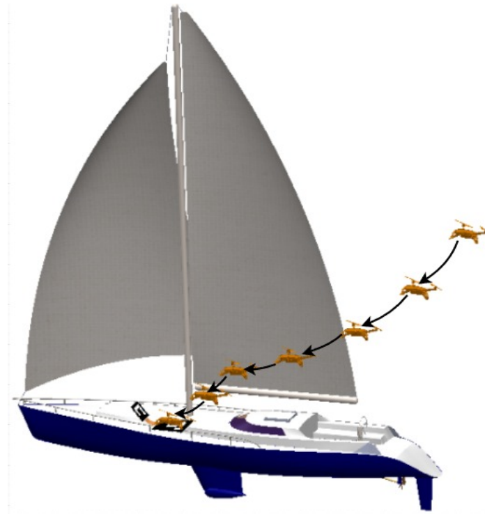
Figure 10. Slide landing: The concept of visual adaptive angle landing of a drone on a moving target. The change in the landing vector is due to the shift of focus from the big target to the small target.
