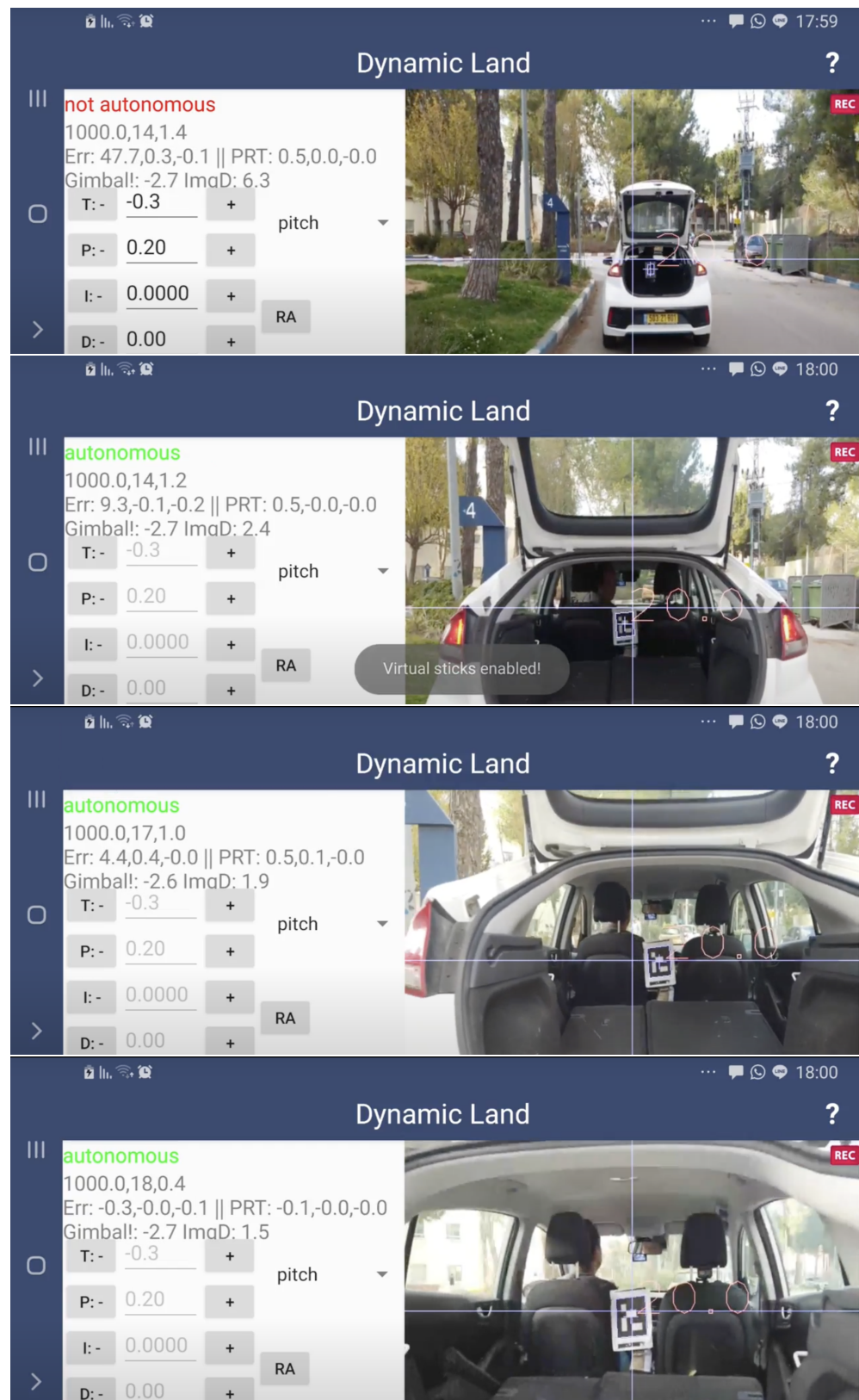
Figure 19. An almost horizontal landing into a moving car (back door). The top image shows the first detection of the landing marker. The second image was taken after the autonomous mode was engaged (see “toast” of a “virtual sticks enabled”). The third image shows the drone maintaining a fixed (leashed) distance and angle from the target, and once this distance is maintained successfully for few seconds, the drone is landing, as shown in the bottom image.
