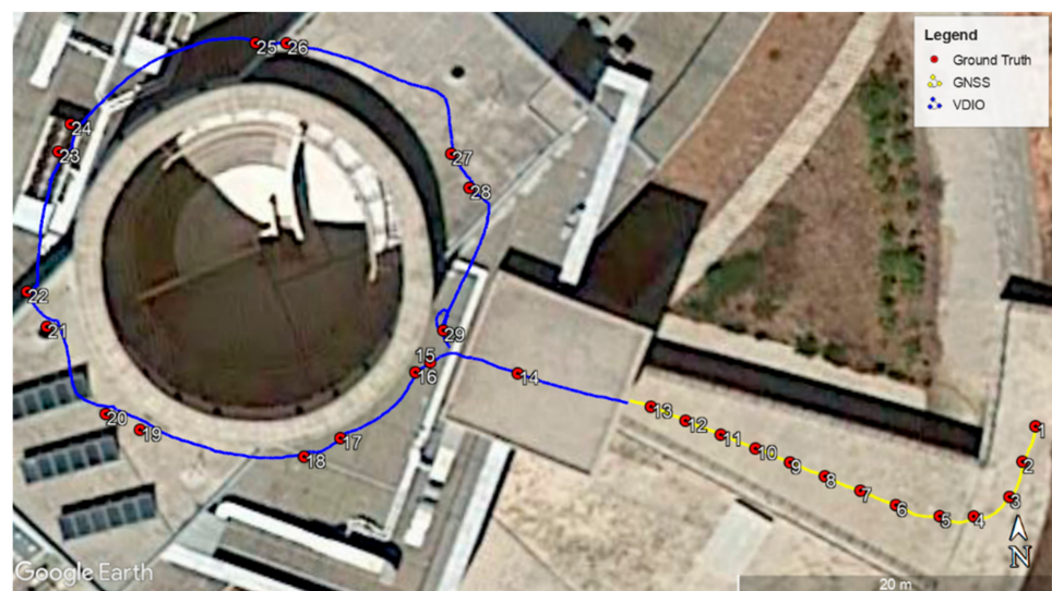
Figure 25. The overall acquired localization output track for the second experiment. This figure indicates the regions where the GNSS-IMU subsystem was selected as the localization source (yellow), as well as the regions where the system handed over the localization task to the vdio_slam (blue).
