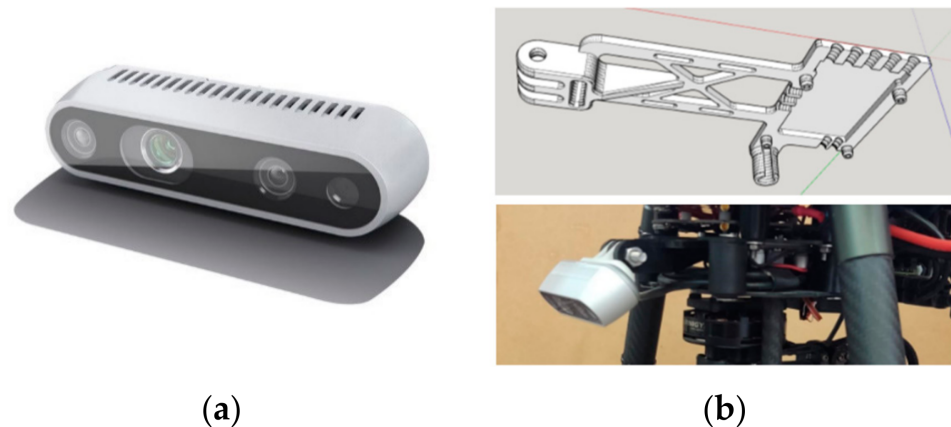
Figure 4. (a) The visual-depth camera sensor Intel RealSense D435. (b) Mounting the D435 onto the aircraft.
