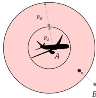
**Figure 5.** Collision definition—breach of a collision region encompassing the combined dimensions of the individual aircraft bodies. Aircraft B enters the collision region volume defined around aircraft A.
