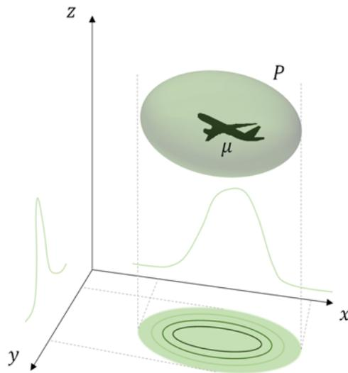
Figure 11. The Gaussian ellipsoid represents the uncertainty in aircraft positioning.
