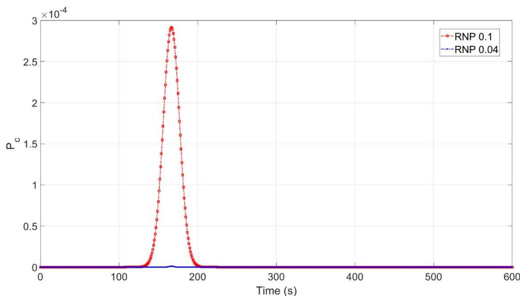
**Figure 21.** Collision risk results for the enroute scenario.
