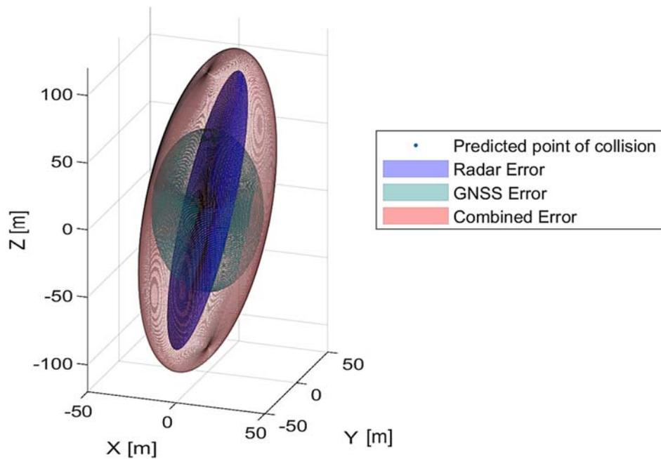
Figure 18. Combined GNSS and Radar Errors.
