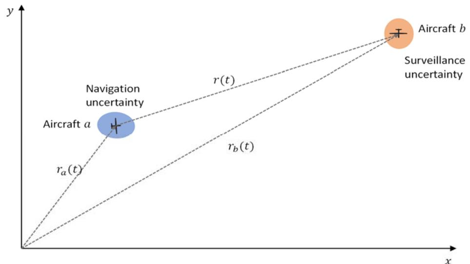
Figure 12. Relative distance as a function of host navigation and intruder surveillance uncertainty.
