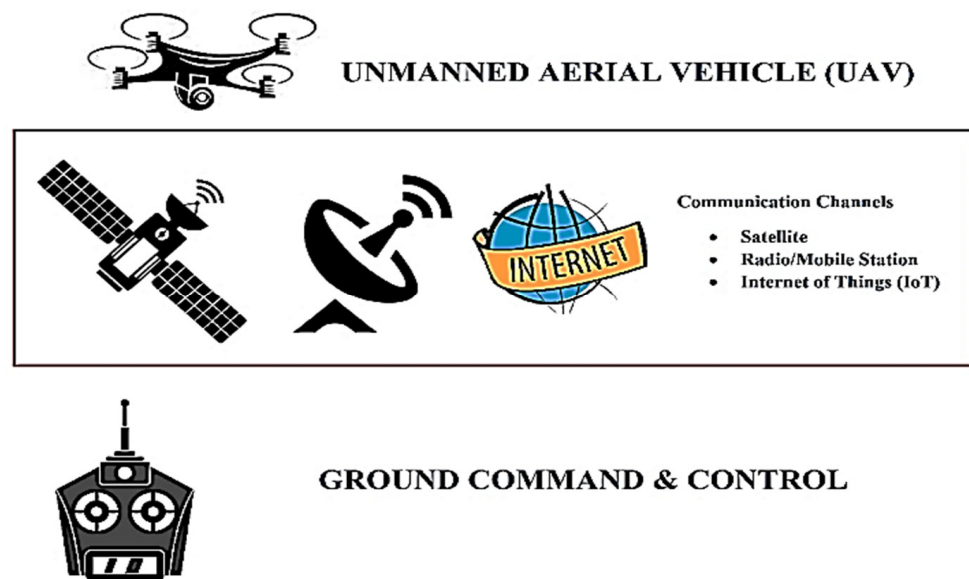
Figure 2. Communication channels mostly used to control UAVs.
