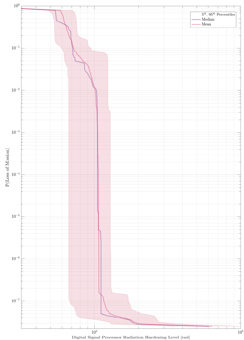
Figure 10. Radiation-hardening targets vs. likelihood of mission failure.
