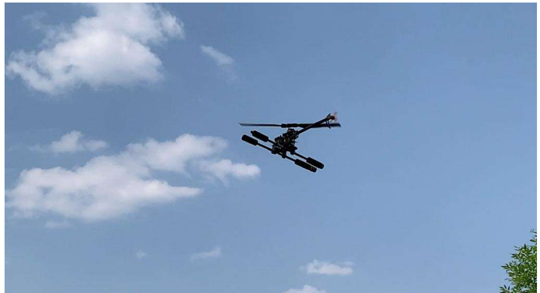
Figure 13. Mini helicopter with virtual swashplate in outdoor hover flight.
