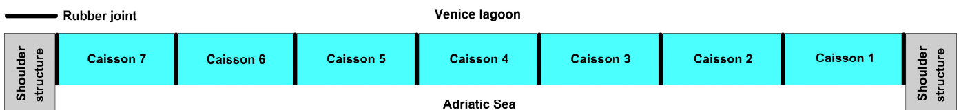
Figure 5. Scheme representing the tunnels that connect the concrete caissons and are protected against flooding by the rubber joints. The shoulder caissons are characterized by emerged structures, whereas the caissons that host the floodgates are submerged and located on the seabed.
