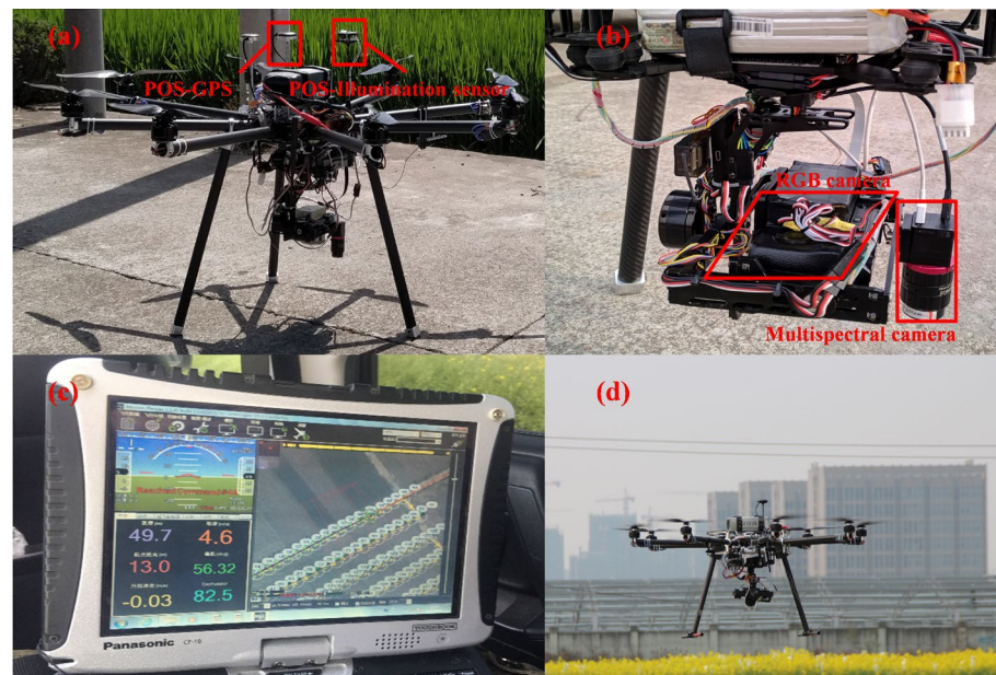
Figure 3. The UAV platform and integrated sensors: (a) POS system; (b) RGB and multispectral imaging sensors; (c) ground control system; (d) flight of the UAV system.
