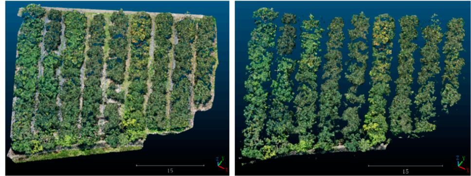
Figure 21. Wipe off point cloud of ground by CSF algorithm.
