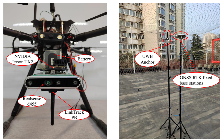
Figure 7. Figure illustrating the outdoor experimental setup, featuring a UAV on the left and the experimental site on the right .
