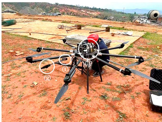
**Figure 17.** Configuration of the UAV-borne cesium optical-pumping magnetometer system integrated with the DJI M600 Pro platform, highlighting key components: ① cesium optical-pumping probe, ② fluxgate sensor, and ③ auxiliary modules (data logger, attitude compensation unit, and RTK/GPS).
