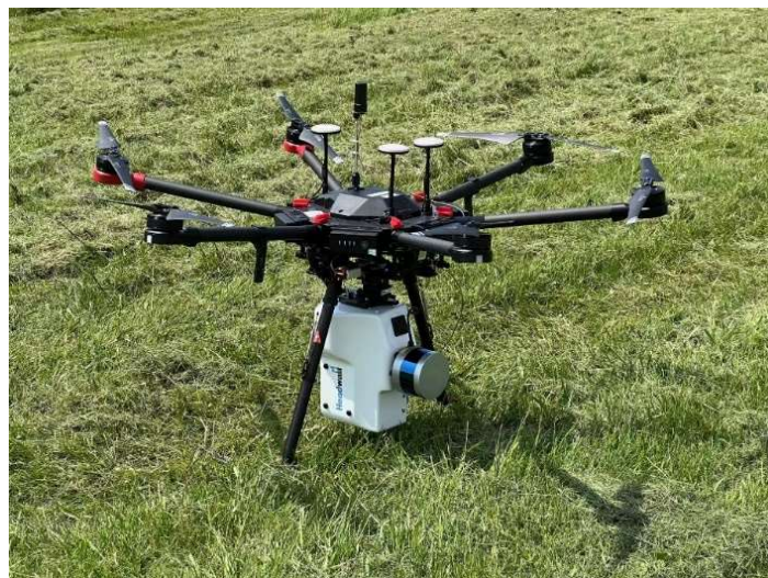
Figure 2. DJI Matrice 600 Pro drone (DJI Technology Co., Shenzhen, China) equipped with a Headwall Hyperspec Co-Aligned VNIR-SWIR Imaging Sensor and a 16-channel Velodyne Lidar Puck (Headwall Photonics, Bolton, MA, USA).
