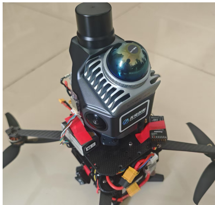
Figure 8. Equipment used for recording datasets. The UAV is equipped with a monocular camera, an IMU, a GNSS receiver, and a LiDAR on its top, where the LiDAR was not used in this experiment.
