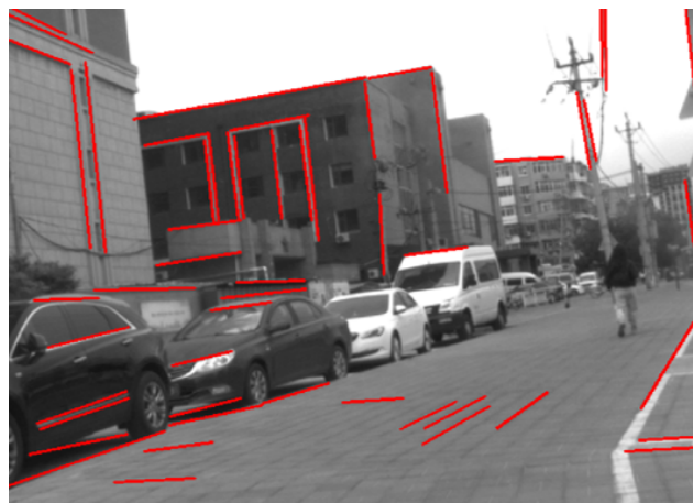
Figure 2. Effect diagram of line feature detection where \eta is set to 0.1. For the frame from the self-collected subway station dataset, short line segments have been filtered out, leaving only the long, easy-to-track line segments.
