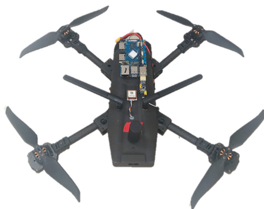
Figure 2. The schematic diagram of the overall external structure of the maize-breeding UAV.
