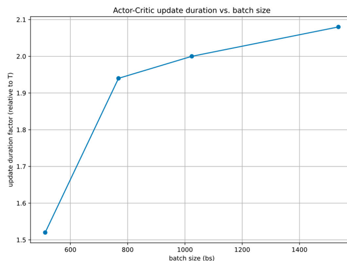
Figure 4. The actor–critic update time (ACUT) duration function of the batch-size, relative to the environment timestep duration. The batch size here is the number of sampled points from the ERB used to update the actor and critic weights. For batch size 512, the ACUT is ~1.5 times the sampling period T_s = 0.1 [s].
