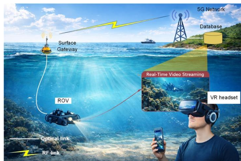
Figure 2. Video streaming through a hybrid communication system used in marine observation, which integrates an underwater drone with a VR headset.
