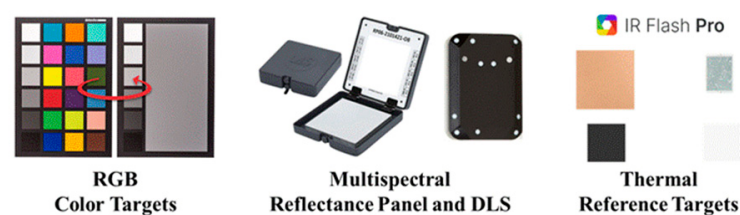
Figure 6. Sensor-specific calibration targets used for image radiometric and reflectance correction, including RGB color checker, multispectral reflectance panel, and thermal reference targets. The thermal references include a black-painted aluminum sheet, a white-painted aluminum sheet, a wooden panel, and an ice–water mixture in an insulated container, representing surfaces with different emissivities and temperatures for thermal calibration.
