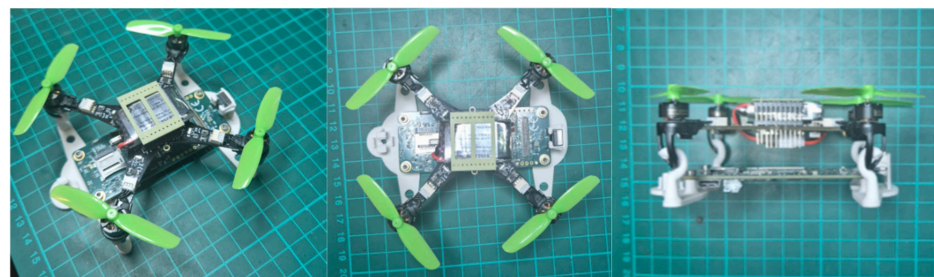
Figure 3. The MCU-EdgeTPU platform mounted on the CrazyFlie Brushless UAV used for the onboard experiments.
