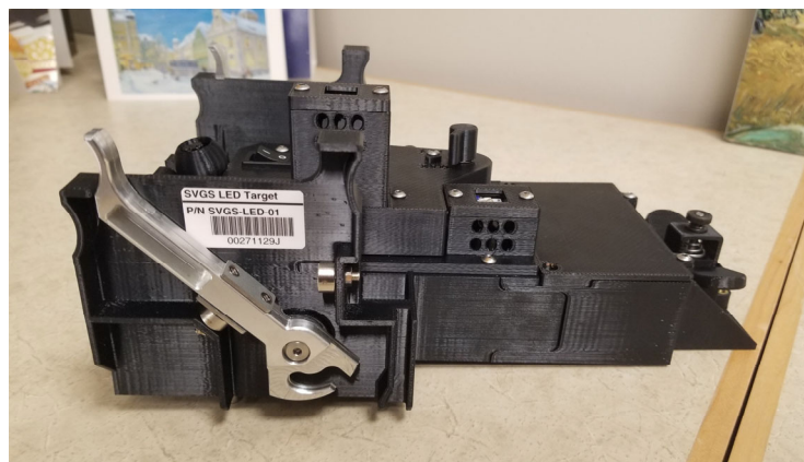
Figure 2. The flight-qualified SVGS tetrahedral beacon (Rev. 8) includes a DC–DC converter, LiPo battery, and overdischarge protection circuitry. A dimmer allows for the adjustment to different illumination conditions within the ISS environment.
