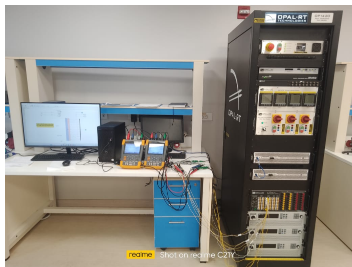
Figure 2. Real-time Hardware-in-the-Loop experimental setup based on the OPAL-RT platform.
