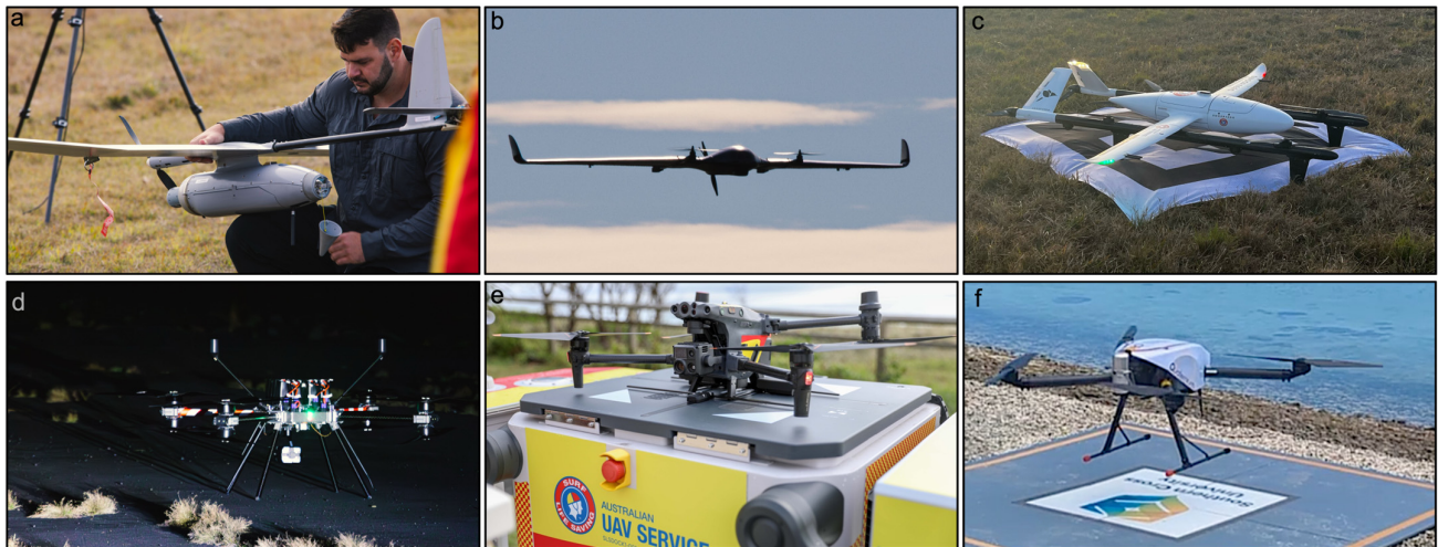
Figure 2. Examples of advanced drone systems with long-range capabilities that have been trialled for shark spotting (a) Elbit Systems of Australia, Skylark I-LEX drone, (b) Flight Technologies, DeltaQuad Pro VTOL fixed-wing drone (c) Swoop Aero Kite VTOL fixed-wing drone, (d) FreeSpace Operations, Calisto 50 heavy lift multirotor drone and (e) DJI Drone-in-a-Box technologies. (f) A Quaternium HYBRiX 2.0 hybrid petrol-electric drone, which has a long flight time (>90 min) for a multi-rotor drone and has been used for coral reef research (Image Credit: (a,b,d,e) Surf Life Saving NSW / Australian UAV Service, (c) K. Monteforte and (f) B. Kelaher).
