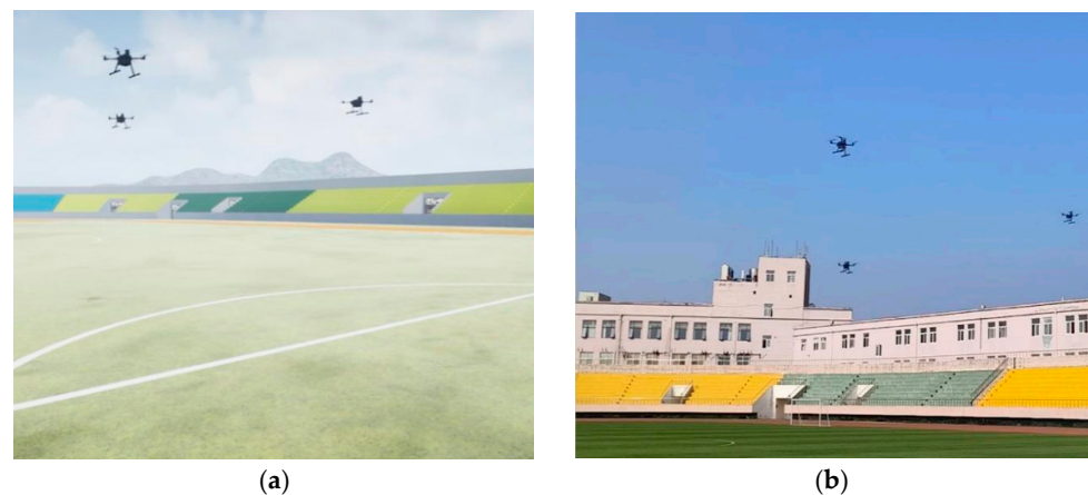
Figure 16. Experimental process of UAV formation flight: (a) digital twin scenario; (b) real-world scenario.
