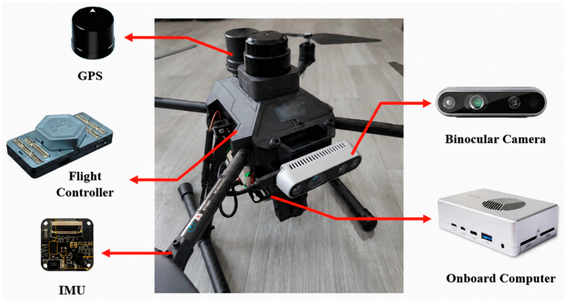
Figure 12. UAV hardware system.
