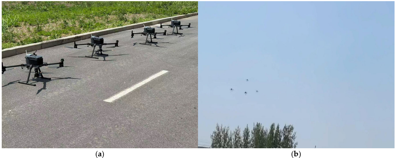
Figure 4. (a) Physical diagram of the UAV platform and supporting equipment; (b) on-site outdoor field test environment. Flight data were collected with this platform and used to build the simulation scenarios; the algorithm evaluation was performed offline in the simulation.
