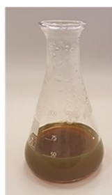
Figure A2. Yellow-green colored solution obtained from the reduction of silver ions by trisodium citrate. Reprinted (adapted) with permission from Abu-Much (2021). Copyright 2021 American Chemical Society.
