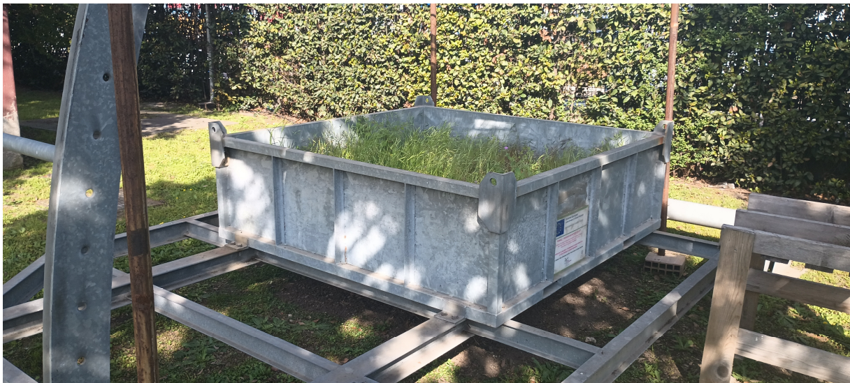
Figure 1. Green roof model.
