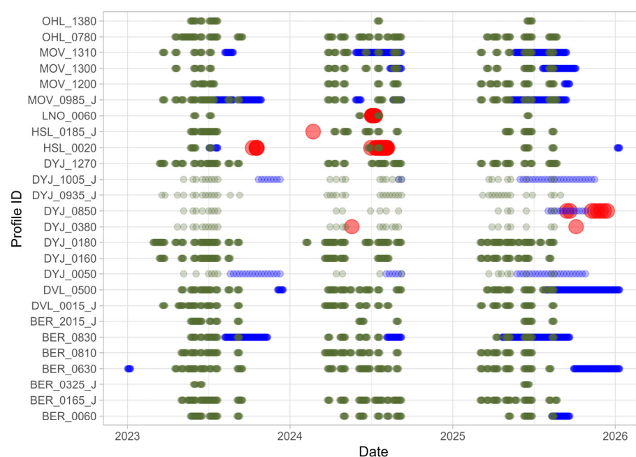
Figure 3. Timing of LTL exceedance (red) in reservoirs compared with SRI (blue) and SPEI (green). Long red clusters indicate sustained operational stress during storage depletion; negative indices can precede breaches or occur without them due to regulation and storage effects.
