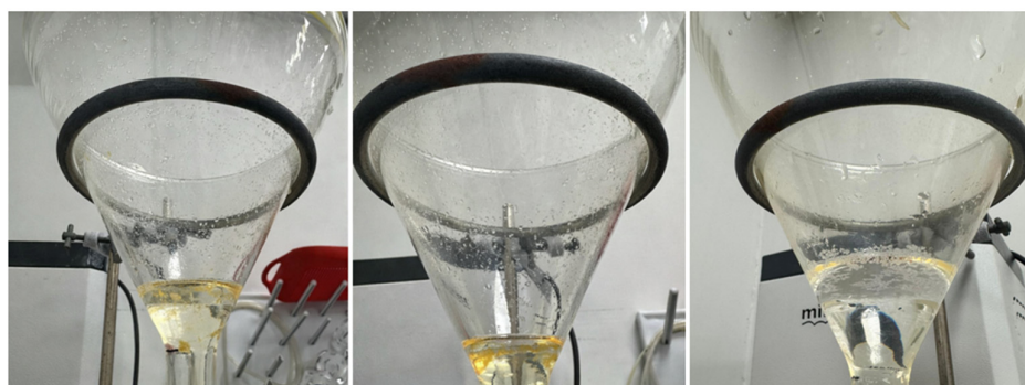
Figure 1. Visual comparison of LDPE behavior during Ives filterability tests. The left cone corresponds to the Tween 20 treatment, the middle cone to the Tween 80 treatment, and the right cone to untreated conditions.
