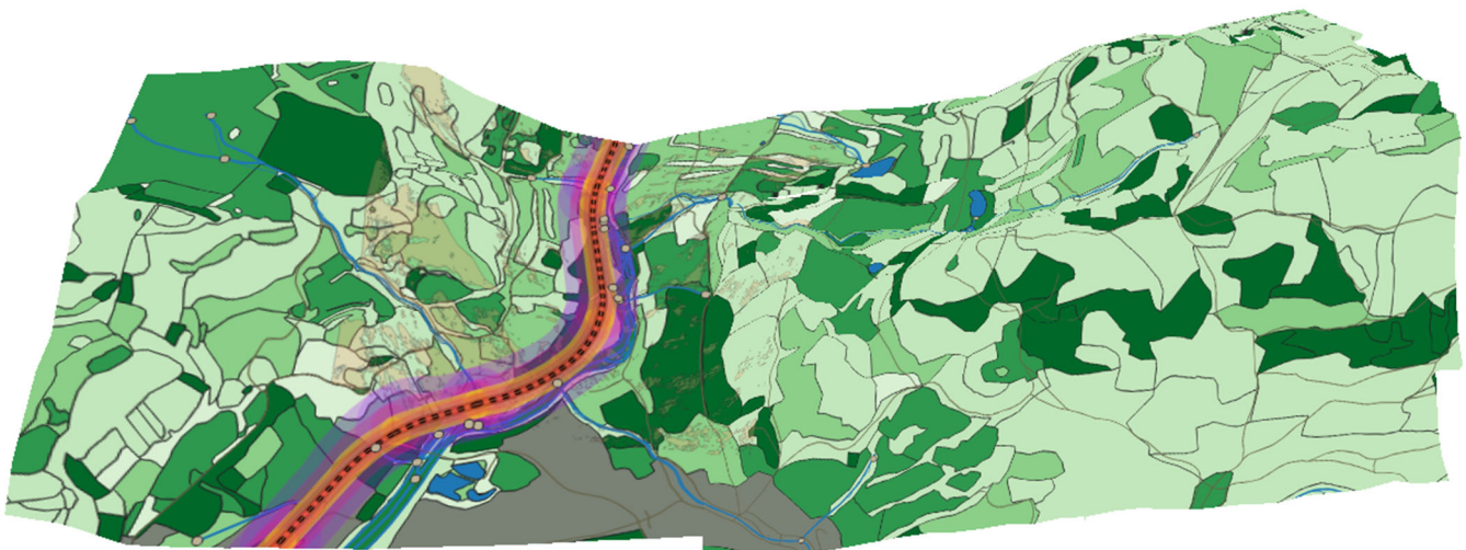
Figure 4. Three-dimensional visualization of the railway corridor and vegetation-management zones. The dashed line represents the railway line, including its vegetation-management/protection zones, running through the centre of the 3D scene. Green polygons in different shades represent areas with different vegetation types. Yellow outlines indicate polygons with cascading fuel structures, while red outlines indicate polygons with potential ladder fuels. Habitat labels were omitted from the figure to improve legibility. However, all vegetation polygons are linked to the GIS attribute database, which enables subsequent vegetation inventory, classification, and further spatial analysis.
