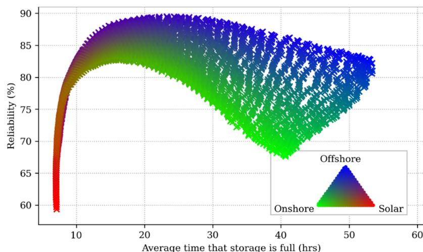
**Figure 6.** A scatter plot showing the reliability of different system designs against the average number of consecutive hours for which the energy storage was fully charged. Each system design has an annual generation of 350 TWh/y and 300 GWh of storage. The colour of the markers indicates relative contribution of each generation technology to the total annual energy generation.
