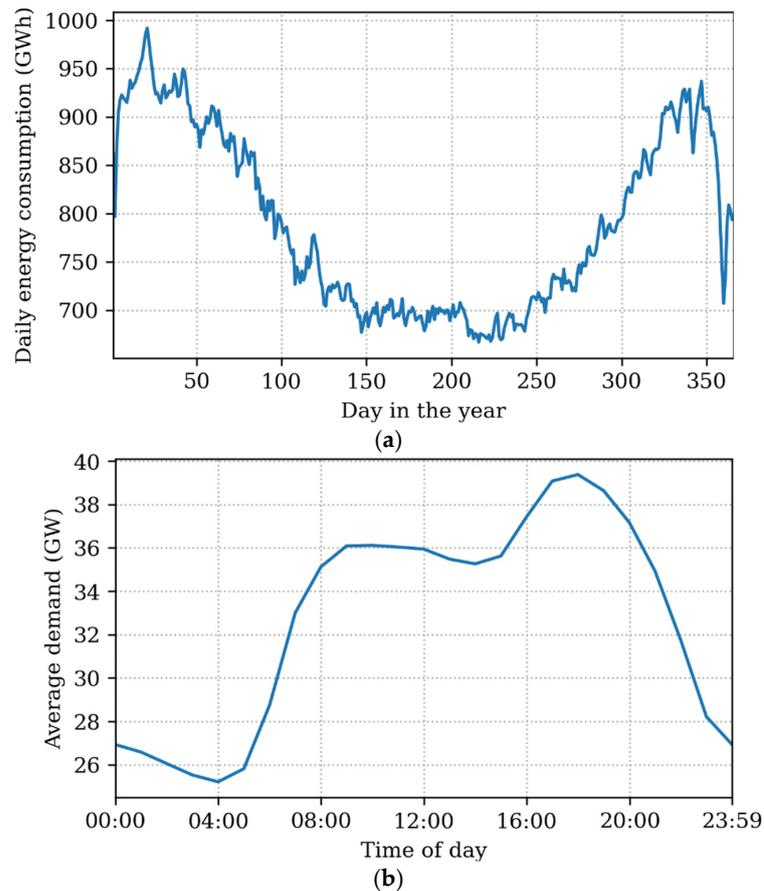
**Figure 2.** Illustration of the electricity demand data used in the simulations: (a) daily electricity consumption throughout the year; (b) electricity demand profile on the “average day”.
