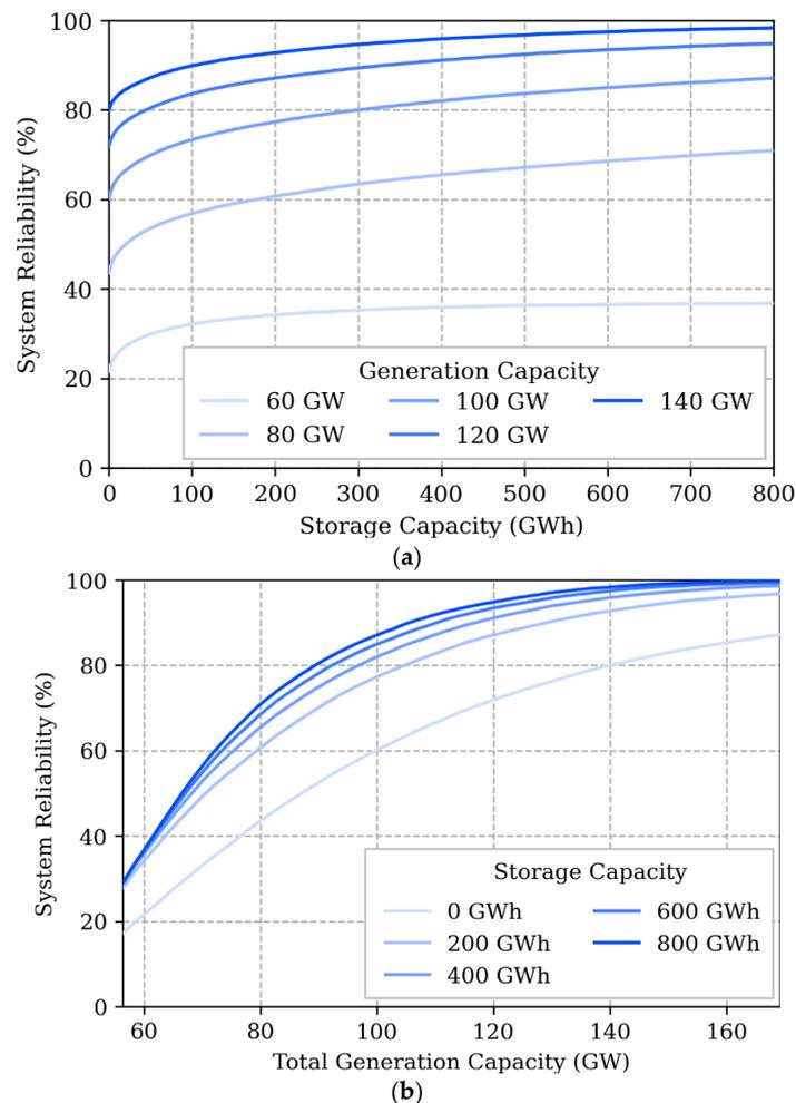
**Figure 3.** System reliability for a range of total system generation and storage capacities: (a) variation in system reliability with storage capacity, for five levels of generation capacity; (b) variation in system reliability with generation capacity, for five levels of storage capacity. Each system is made up of 40% offshore wind, 30% onshore wind and 30% solar PV.
