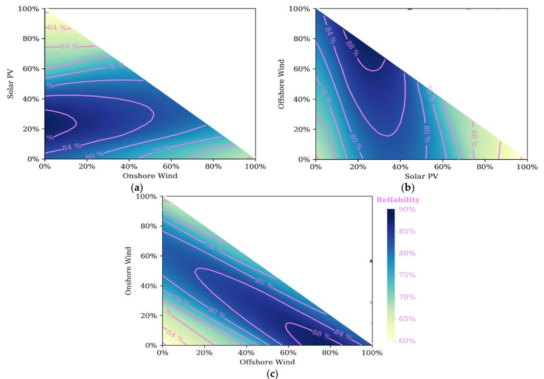
**Figure 5.** System reliability as a function of renewable energy generation mix of solar PV, offshore wind and onshore wind with a fixed annual generation of 350 TWh/y and a fixed storage installed capacity of 300 GWh. Graph (a) shows reliability of mixtures of offshore wind and solar PV, Graph (b) shows reliability with mixtures of solar PV and onshore wind and Graph (c) shows reliability with mixtures of onshore wind and offshore wind.
