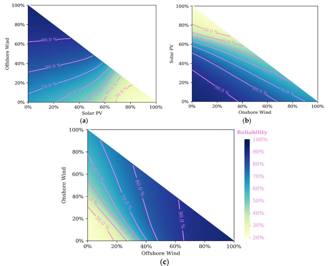
**Figure 4.** System reliability as a function of renewable capacity generation mix of solar PV, offshore wind and onshore wind with a total installed capacity of 100 GW and a fixed storage installed capacity of 300 GWh. Graph (a) shows reliability of mixtures of offshore wind and solar PV, Graph (b) shows reliability with mixtures of solar PV and onshore wind and Graph (c) shows reliability with mixtures of onshore wind and offshore wind.
