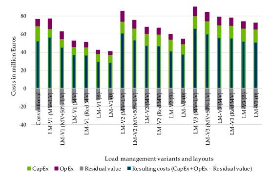
**Figure 17.** Consolidated costs over eleven medium voltage grids for conventional planning strategy and three load management variants with six layouts based on [59].
