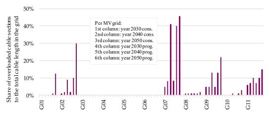
**Figure 20.** Share of the length of overloaded cable sections to the total cable length in the grid for the two development scenarios over three years until 2050 based on [59].
