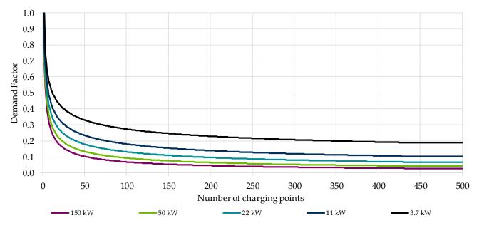
**Figure 2.** Demand factors for five dominant charging powers for up to 500 charging points based on [50].
