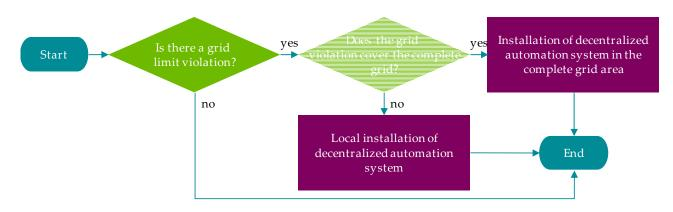
**Figure 5.** Flowchart for the installation of the components of the decentralized automation system for applying load management based on [59].
