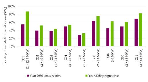
**Figure 16.** Loading of substation transformers for 9 medium voltage grids in the year 2050 for the two development scenarios.
