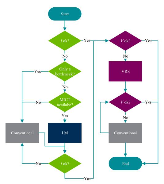
Figure 22. Flowchart for planning medium voltage grids.
