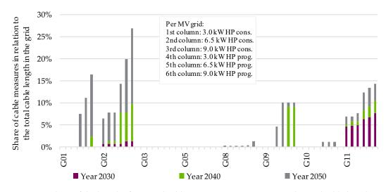
**Figure 19.** Share of the length of required cable measures in comparison to the total cable length in the grid for the two development scenarios over three years until 2050 based on [59].
