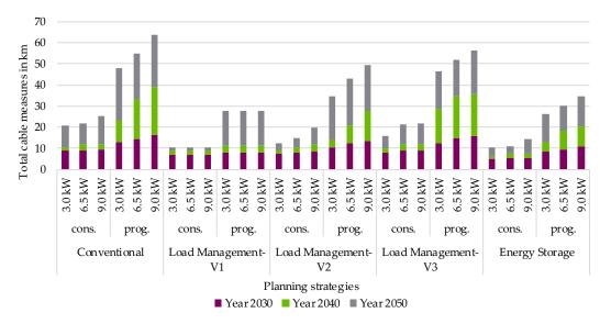
**Figure 9.** Consolidated cable measures for the medium voltage grids with different planning strategies over the investigated years for the two development scenarios and the three heat pump systems.
