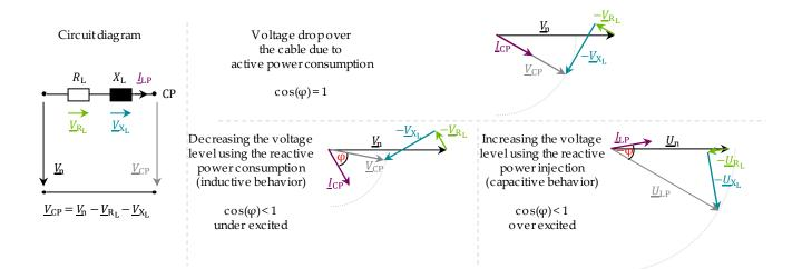
Figure 7. The principal operation of reactive power management based on [59].
