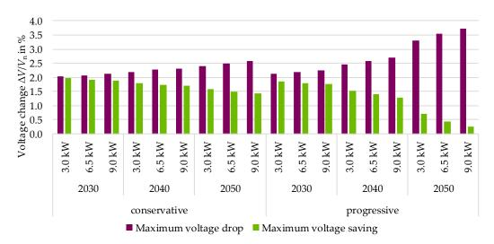
**Figure 21.** Maximum voltage drop and maximum voltage saving consolidated over eleven MV grids for the two development scenarios over three years until 2050 based on [59].
