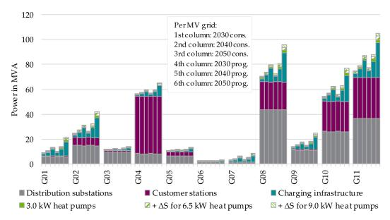
**Figure 8.** Load development for eleven medium voltage grids for the two development scenarios over the years 2030, 2040 and 2050 based on [59].
