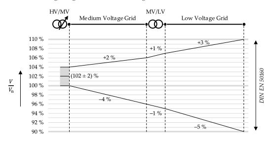
Figure 4. Assumed division of voltage range between medium voltage and low voltage grids.
