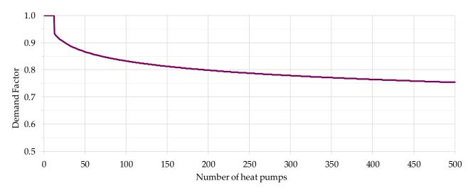
Figure 3. Demand factors for up to 500 heat pumps based on [51].
