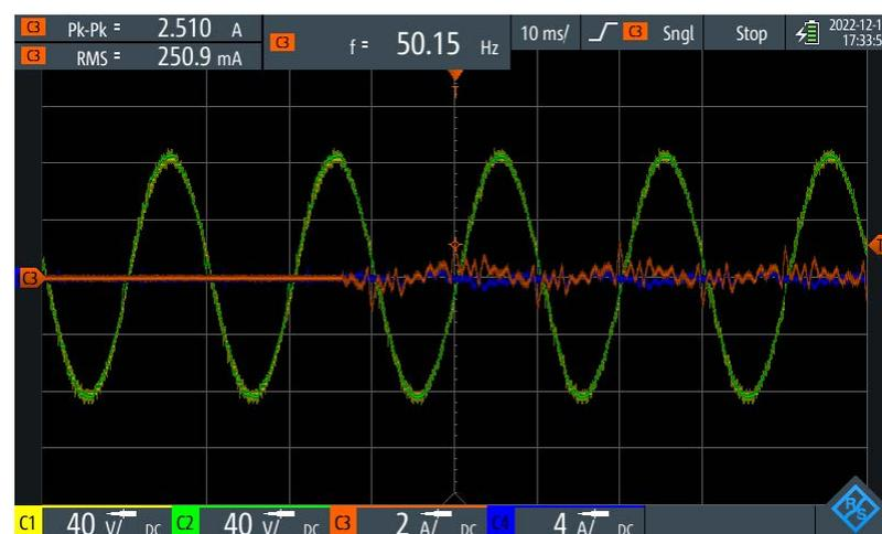
**Figure 8.** System parameters at operation startup with a  $V_{\text{grid}}$  of 56 V RMS,  $I_{\text{sys}}$  of 0 A RMS and  $f_{\text{grid}}$  of 50 Hz. Grid voltage (green), inverter voltage (yellow), inverter current (red) and current of a single battery cell (blue).
