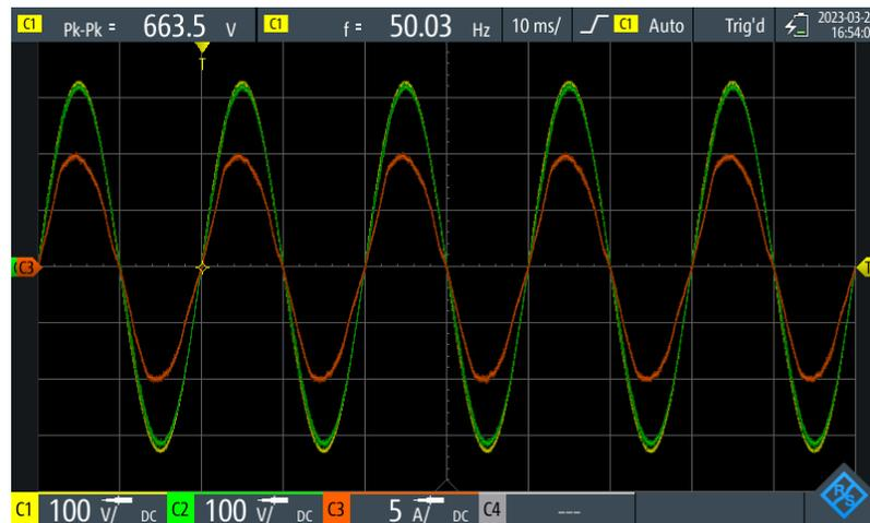
**Figure 9.** System parameters at operation with a grid voltage of  $V_{\text{grid}}$  230 V RMS, a system charging current  $I_{\text{sys}}$  of 7 A RMS and a grid frequency  $f_{\text{grid}}$  of 50 Hz. Grid voltage (yellow), system voltage (green) and system current (red).
